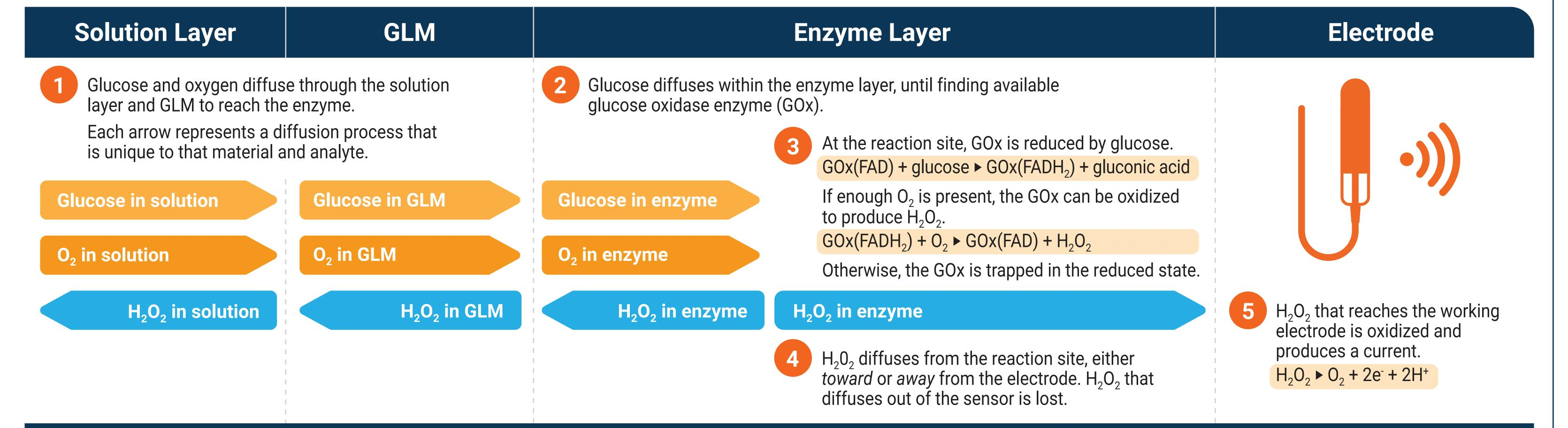
**Sensor response and linearity** are affected by the balance of glucose and  $O_2$  within the sensor, and the fraction of  $H_2O_2$  that is detected at the electrode surface. Sensor response time is affected by the rate of diffusion of each analyte through various materials.
